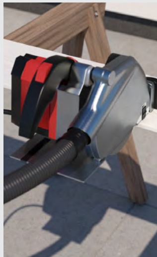
When using the Hardie™ Blade sawblade, most circular saws will require the painted face of the boards to be downward facing. We advice this to be double checked prior to cutting.
